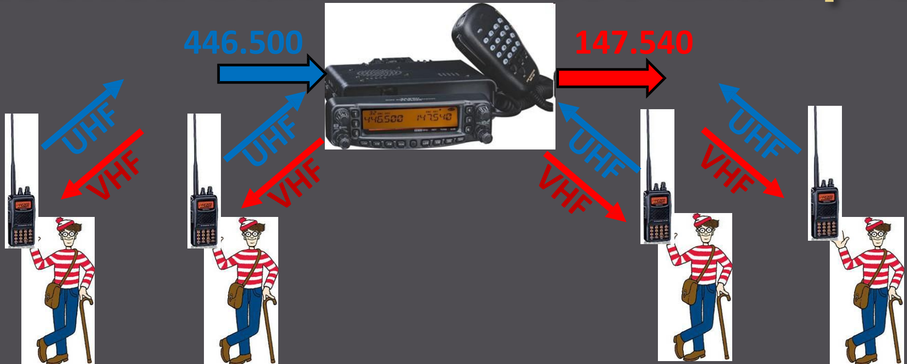
Locked Band Radio Field Repeater
